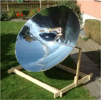
It is a solar cooker with a parabolic reflector of just over 1 m<sup>2</sup> of caption area, which corresponds to a theoretical output of about 1 kW. The production requires several materials and quite skilled craftsmanship in dealing with these materials and tools. It must be worked exactly, therefore, all the dimensions of this construction manual are given in millimeters.
